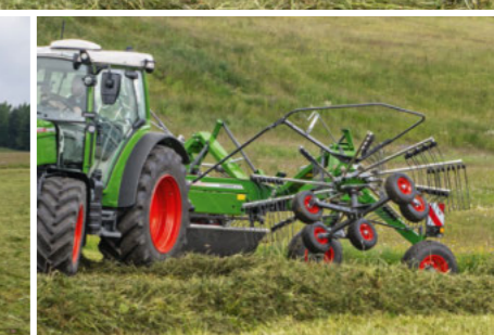
The swath curtain folds up automatically in the headland or transport position
