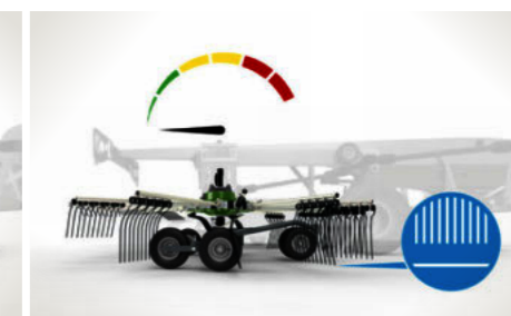
3 Standstill All four rotors raise the tines above the pre-set clearance height.
