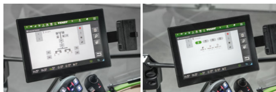
ISOBUS UT: transfer user screens to the tractor terminal ISOBUS AUX-N: option for joystick controls to take over
