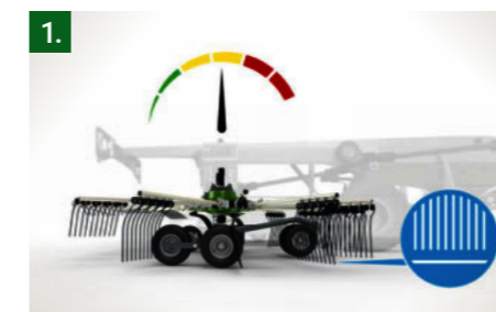
1 Start-up All four rotors lower to the preset raking height.
