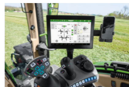
ISOBUS UT: Operating screens can be transferred to the tractor terminal ISOBUS AUX-N: Control lever transfer is possible
