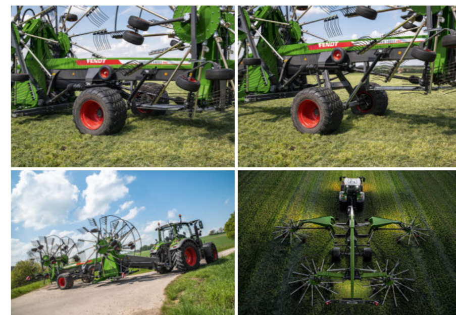
Intelligent towing hitch: The angle sensor warns if the hitch is too tight.
