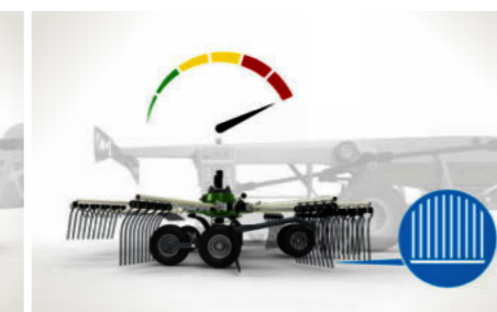
2 Increase driving speed All four rotors lower below the preset raking height depending on the driving speed.
