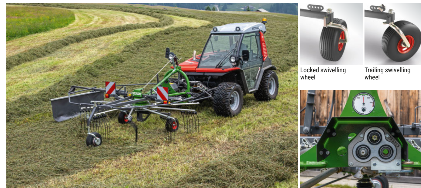
Universal transmission made of cast light metal for front and rear operation.
