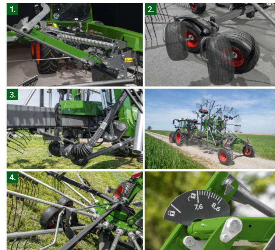
The raking height is set quickly and easily using a winding handle on standard models and hydraulically on PRO models
