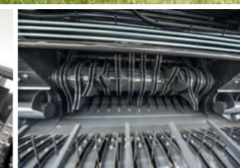
XtraCut13 Rotor (Finger pair distance: 90 mm) - Without cutting system (series) - With cutterbar: up to 13 knives
