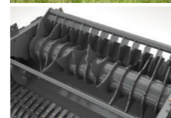
Conveyor rotor without cutting system
