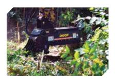
Digga's Flail Mower for Excavators up to 10 tonnes has been engineered to handle your toughest vegetation management jobs.
