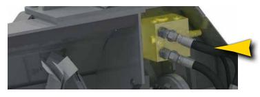
Bi-directional flow manifold with cross-over relief allows the operator to direct debris away from bystanders, other machinery, and buildings
