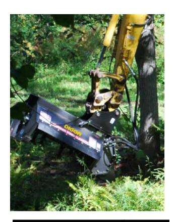
SPECIFICATIONS 760mm / 30" 1000mm / 40" Model Overall Width 813mm 1065mm **Cutting Width** 724mm 975mm **Cutting Capacity** 100mm 100mm Depth 750mm 750mm 60-85 120-150 Hydraulic Flow (LPM) Machine Suitability 3 to 6t 6 to 10t Case Drain Required Yes Yes 240 345 Pressure (BAR) 1800-2200 Rotational Speed (RPM) 1800-2200 Weight 380kg 533kg **Blade Stands** 8 10
