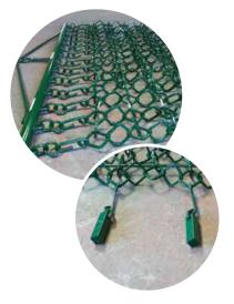
**TOP:** Chain mesh section **BOTTOM:** Weights used to retain shape
