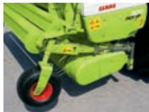
Hydraulically folding castor guide wheels
