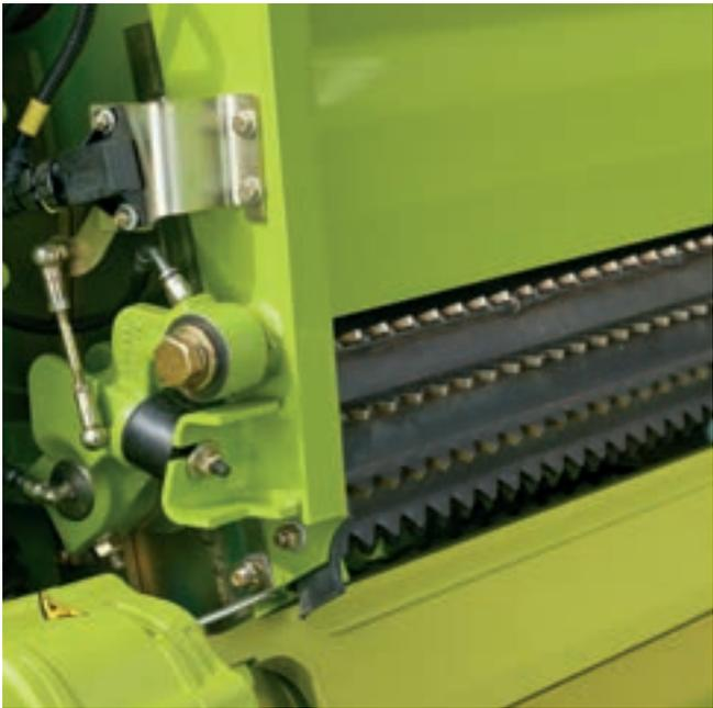
Throughput measurement with the QUANTIMETER.
