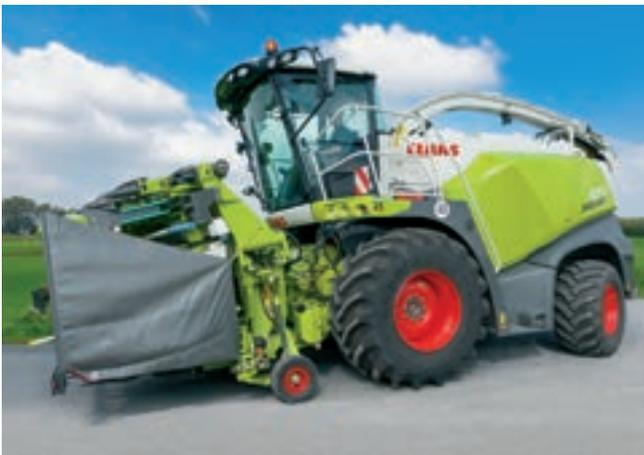
NEW: Integrated transport system. During road travel, the running gear integrated in ORBIS is deployed. The hydraulic rams are actuated actively during road travel. The vibration damping allows comfortable and safe road travel at up to 40 km/h.
