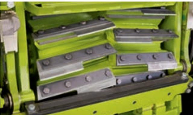
The chop length can be doubled by equipping the V-CLASSIC cylinder with half-knives. The half-knives enable a very consistent crop throughput which is ideal when harvesting grass or maize for long chopping and SHREDLAGE.
