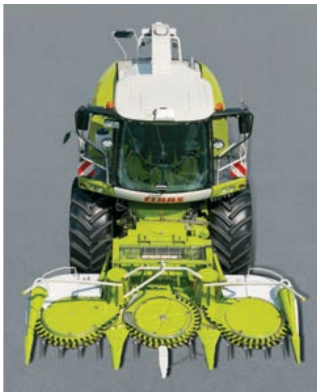
An aggressive crop flow is ensured by the intake auger whose speed can be optimised in line with the set chopping length. The simple construction makes for ruggedness and reliability and has proven itself remarkably well.
